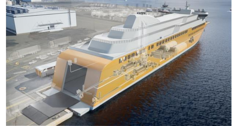
Hybrid propulsion (400 MWh batteries)
